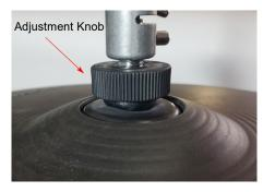
This knob allows you to adjust how much pressure is required to have to pedal register completely closed. Turning clockwise makes it more pressure sensitive and turning it anti-clockwise makes it less pressure sensitive.
